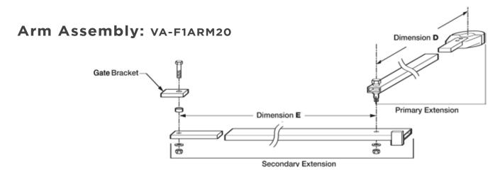
⚠ IMPORTANT: When attaching the Arm Assembly to the gate, if the "Gate Bracket" is not welded to a frame member that runs the full length of the gate, the operator may damage the gate. Do not attach the Gate Bracket to only a few pickets.
