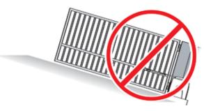
DO NOT install the gate operator to lift gates
