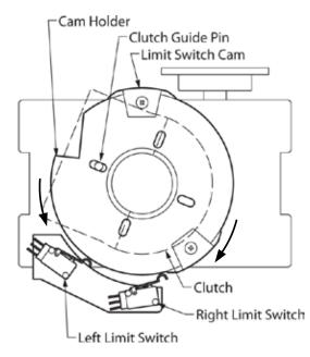
**Tip:** Referring to Step 2b. The "Cam Holder" contains four (4) Guide Pin holes to allow for proper positioning, if required, due to an alternative operator orientation.
