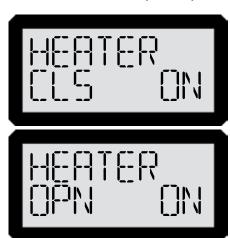
**NOTE:** If the application requires the gate to be held open for any reason, set the HEATER ON for both limit positions.
