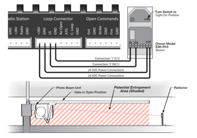
Consult the installation manual for the UL325 device (photo beam or like) for detail information about the usage, installation and maintenance.
